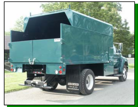
UTV Body – features removable side walls and roof.
